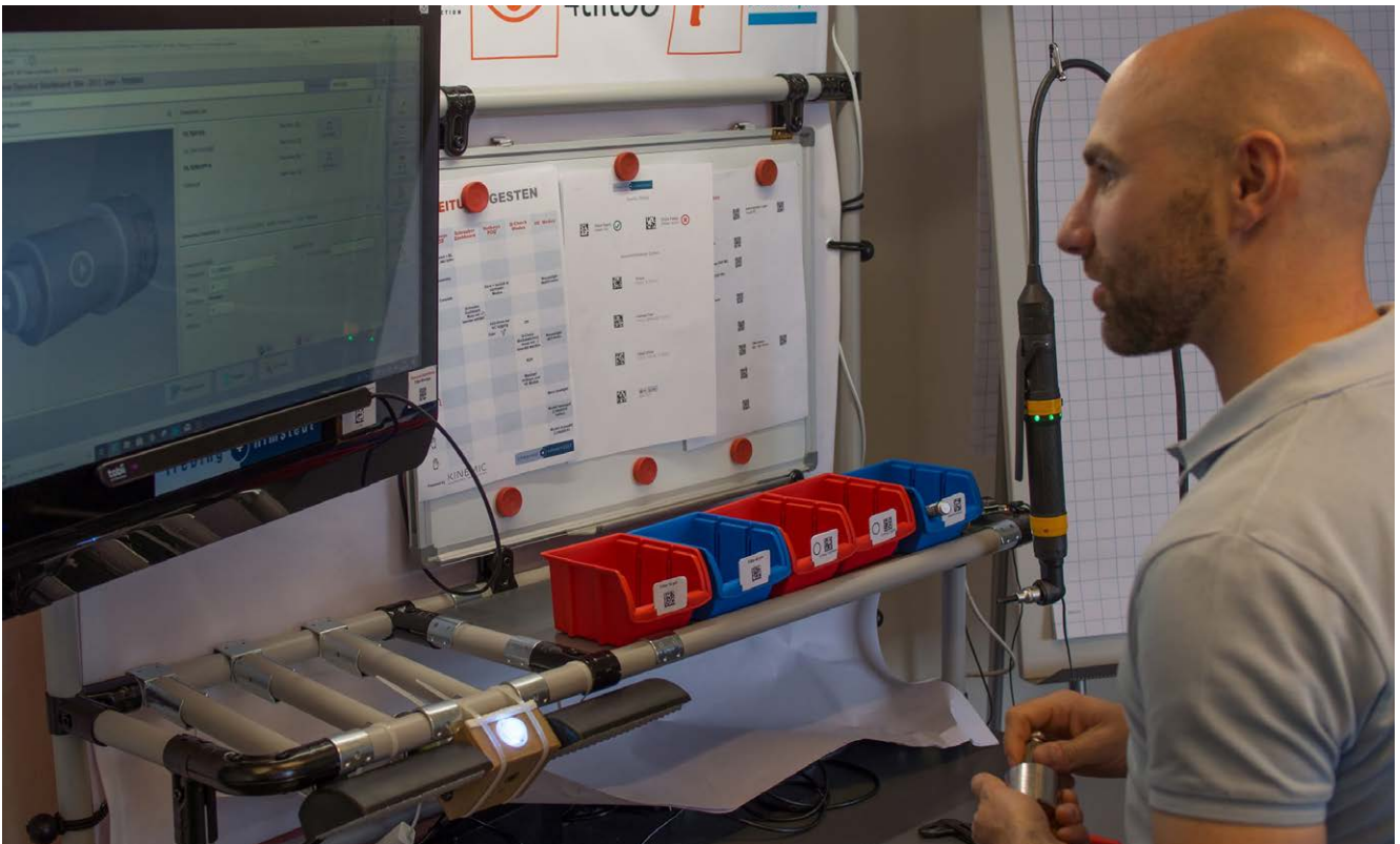
An operator uses gaze and gestures to navigate through an SAP assembly assistance system
