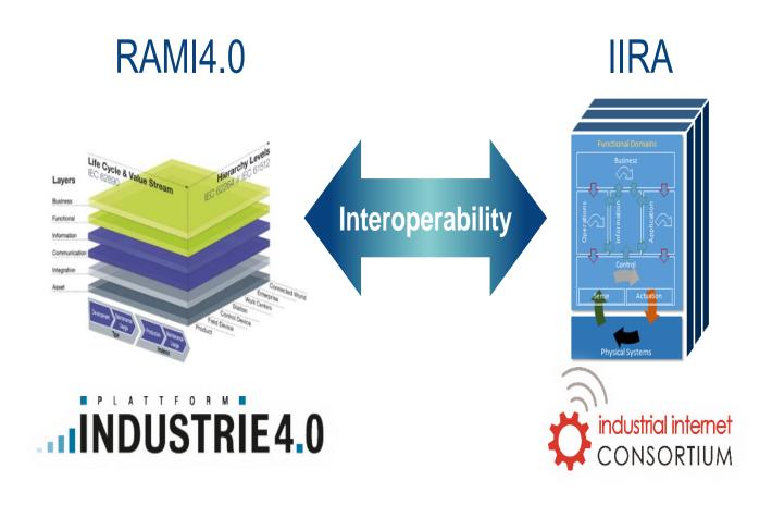
The IIC and Industrie 4.0 are working together to map architectures and provide eventual interoperability. A key part of that mapping is to understand and map the "connectivity" communications layer.
